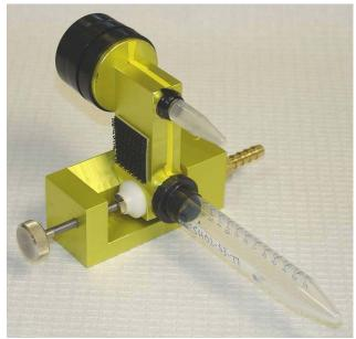
The calibration adaptor is shown here with a BC 221 sampler (left) and a BC 251 sampler (right) properly inserted.
