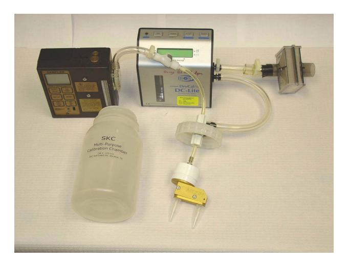
**Flow calibration.** The airflow through the sampler must be calibrated before each use. A calibration jar may be used for this purpose. SKC makes a large calibration jar (#225-112) that will fit all of the samplers, including the BC 251. Attach the sampler to the fitting as shown and place it in the jar. Connect the pump and flow meter. Turn the pump on and allow it to warm up for 5 minutes before setting the flow rate.
