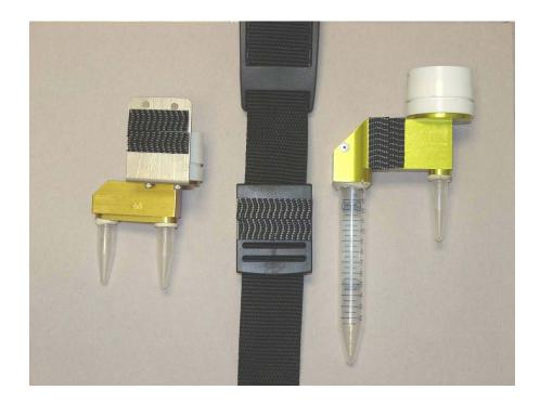
Samplers and buckle showing black Dual Lock strips. When the noise-reducing cases are used, the sampler is mounted on a buckle on the case shoulder strap. To mount the sampler on the buckle, press the sections of Dual Lock strip together. Pull them apart to remove the sampler. The buckle is on the shoulder strap for a noise-reducing case. It can be moved along the strap as needed, and can be pried apart and moved to a different part of the strap if necessary.
