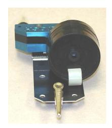
BC 221 sampler: The tubes and filter cassette on the BC 221 are sealed with tape as shown rather than caulk. The seam around the sampler is sealed with tape to prevent air leakage during use. The filter cassette is black to help hold the sampler more conductive polypropylene.
