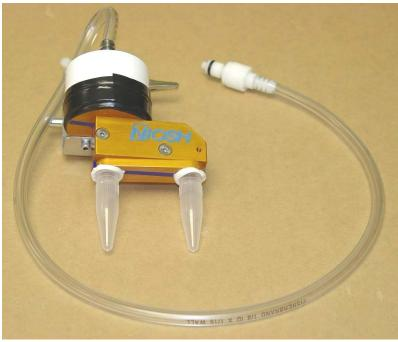
Assembled two-stage BC 212 sampler: White material at top of Eppendorf tubes is rope caulk for sealing. Blue tape on sampler seals the seam where the two halves join together. Black tape around the filter cassette helps keep the cassette in place and seals any possible leaks. A Luer fitting plugs into the top of the filter cassette. 1/8" ID tubing connects the Luer fitting to a CPC quick-disconnect fitting
