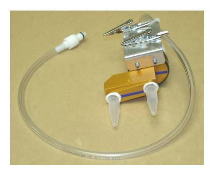
Rear view of BC 212 sampler: The stainless-steel L-bracket allows the sampler to be clipped onto a worker. This bracket attaches with two socket-head screws as seen. The bracket can be removed if it is not needed. The bracket has four holes for alligator clips (two clips are shown). The clips can be rotated or moved to different holes as desired.
