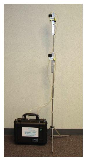
Two NIOSH samplers are shown on a tripod in a healthcare facility. The black case on the floor contains two sampling pumps that pull air through the samplers.
